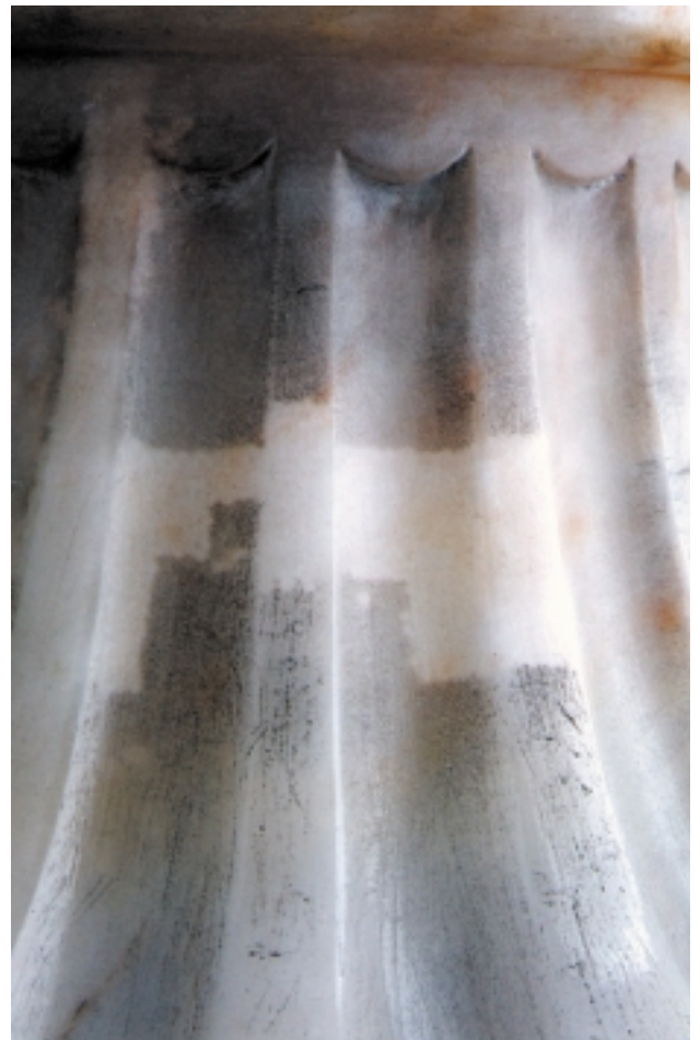
Figure 4 Fragment of a laser-cleaned alabaster flower-pot.
